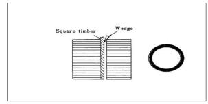
g) In no case should the drums be stored 'on the flat that is, with flange horizontal. Cable drum should always be stored and transported standing on both flanges. They should not be pushed along the ground standing on the flanges. It is possible that the strength of the cable drum would then no longer be guaranteed.
