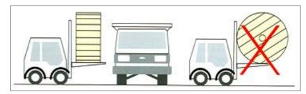
k) Unloading the drum should be by forklift or crane, rolling should be avoided.
